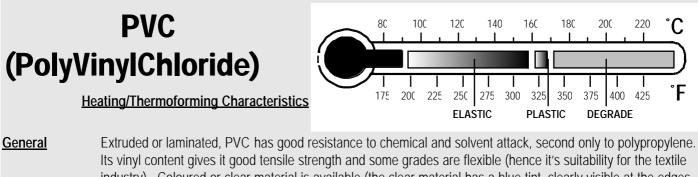
industry). Coloured or clear material is available (the clear material has a blue tint, clearly visible at the edges of sheets). Resistant to water and fire (as it burns it releases chlorine atoms which inhibit combustion) and reasonably impact resistant, it is the leading TP in the construction industry.
