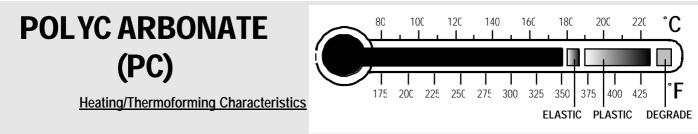
**General** A dense TP with high impact resistance and superior fire rating, available in a number of forms and sections, including sheets. Limited colours, clear, smoke shades plus a variety of embossed textures. Good weather and UV resistance, with transparency levels almost as good as acrylic.
