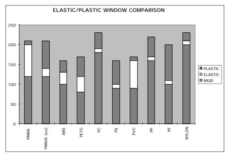
The temperatures at which TP's become elastic or plastic depend on the material type.
