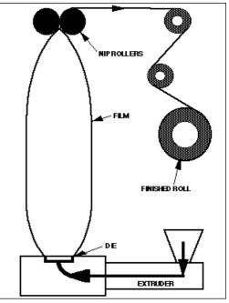
extrudate, through the die and onto the rollers, has been established, air is blown into the tube at the point at which it leaves the die - when it is still pliable - to expand it to the required size. This film tube is flattened, cooled and loaded onto its final reel by the roller system.
