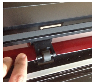
After your cutting session, trim off your vinyl straight across by cutting with an Xacto knife. Drop your blade into a horizontal channel and pull it across, cutting both the vinyl and the paper.
