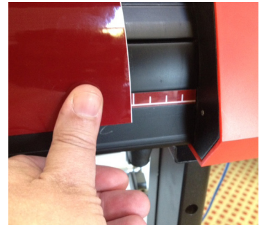
When loading vinyl, make sure you use at least 2-3 clamps and center them under the white brackets.
