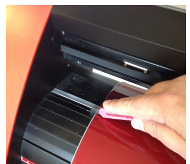
After your cutting session, trim off your vinyl straight across by cutting with an Xacto knife. Drop your blade into a horizontal channel and pull it across, cutting both the vinyl and the paper.
