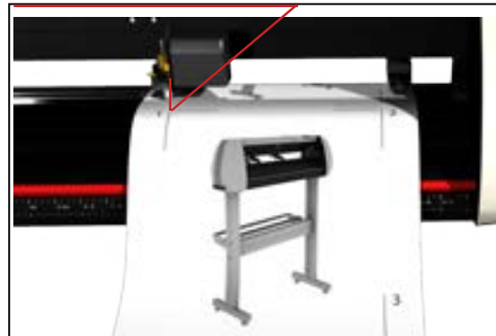
Laser centered on registration dot
